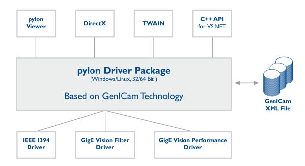
The internal architecture of the pylon driver package is based on GenlCam Technology, which offers you easy access to the newest camera models and the latest features. Changes to an existing camera device in your application essentially become a plug-and-play process.
