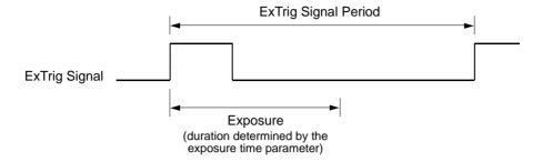
Fig. 45: Timed Exposure with Rising Edge Triggering
