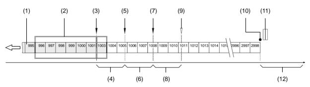
Fig. 30: Combination of Threshold Resend Mechanism and Timeout Resend Mechanism
