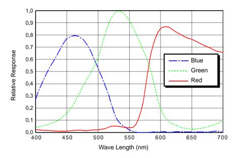
Fig. 11: scA640-70gc Spectral Response
