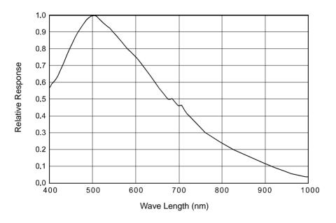
Fig. 10: scA1600-14gm Spectral Response
