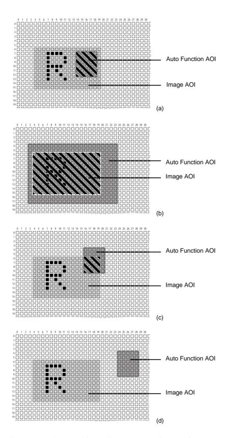
Fig. 70: Various Degrees of Overlap Between the Auto Function AOI and the Image AOI
