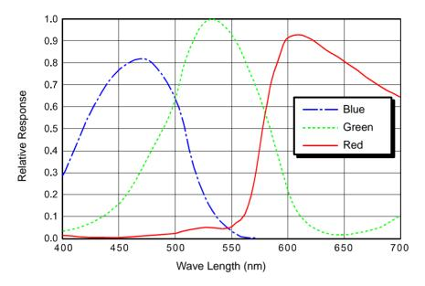
Fig. 12: scA640-74gc Spectral Response
