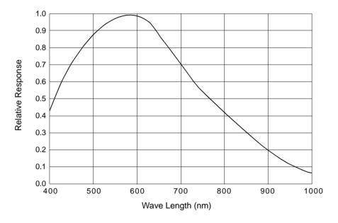
Fig. 7: scA1300-32 gm Spectral Response
