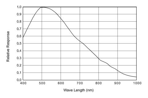
Fig. 2: scA640-74gm Spectral Response
