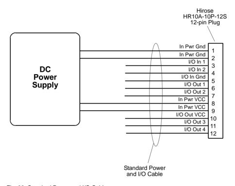
Fig. 38: Standard Power and I/O Cable
