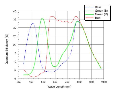
Fig. 14: scA750-60gc Spectral Response
