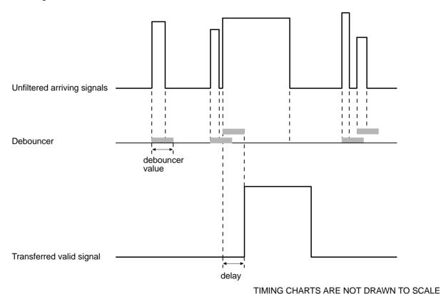
Fig. 71: Filtering of Input Signals by the Debouncer
