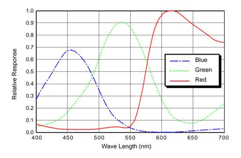
Fig. 17: scA1300-32gc Spectral Response
