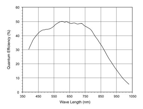
Fig. 4: scA750-60gm Spectral Response
