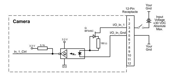
Fig. 39: Typical Input Circuit
