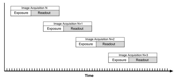
Fig. 49: Overlapped Exposure
