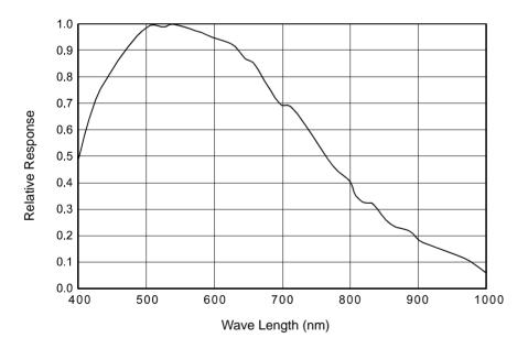
Fig. 9: scA1400-17gm and scA1400-30gm Spectral Response
