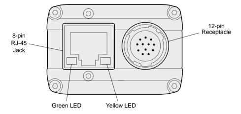
Fig. 36: Camera Connectors and LED
