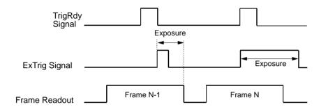
Fig. 47: Trigger Width Exposure Mode with Overlapped Exposure
