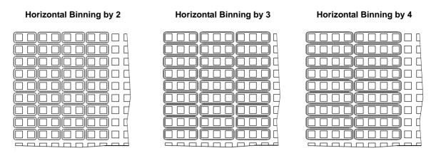
Fig. 62: Horizontal Binning
