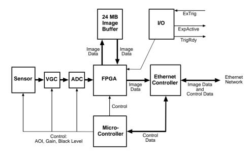
Fig. 33: Camera Block Diagram
