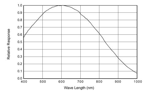
Fig. 3: scA640-120gm Spectral Response
