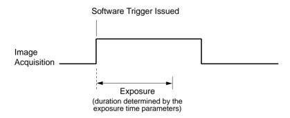
Fig. 44: Image Acquisition with a Software Trigger
