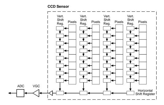
Fig. 32: CCD Sensor Architecture
