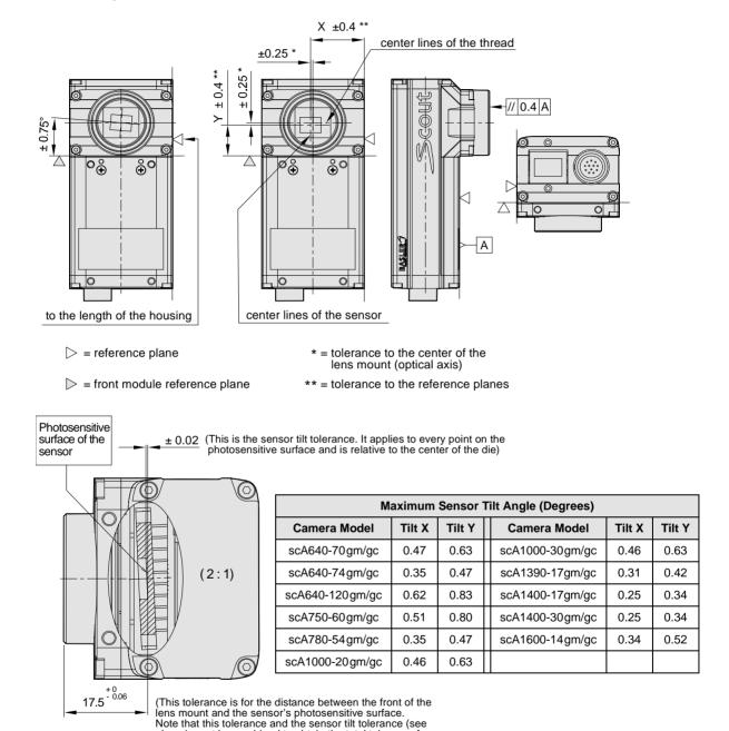
Fig. 26: Sensor Positioning Accuracy for Cameras (90° Head) with the Standard C-mount Lens Adapter (in mm unless otherwise noted)
