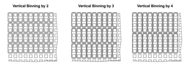
Fig. 61: Vertical Binning
