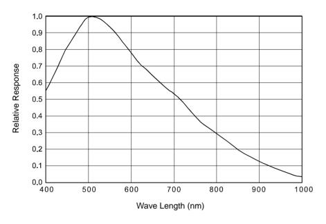
Fig. 6: scA1000-20gm and scA1000-30gm Spectral Response
