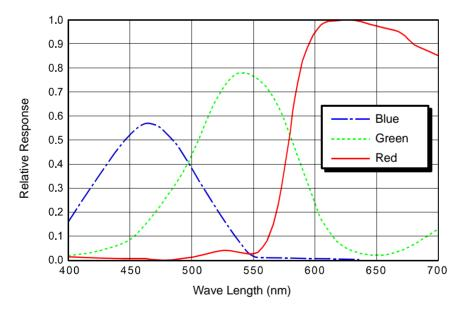
Fig. 13: scA640-120gc Spectral Response
