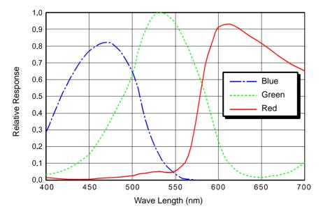
Fig. 15: scA780-54gc Spectral Response
