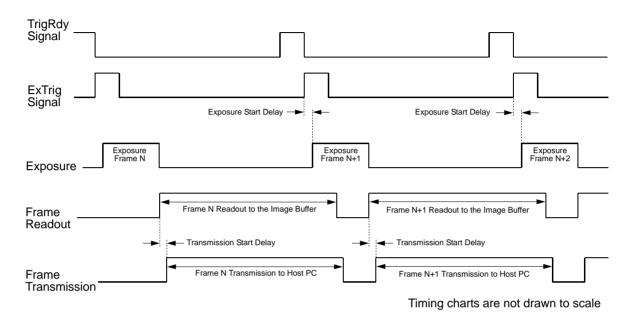
Fig. 54: Exposure Start Controlled with an ExTrig Signal
