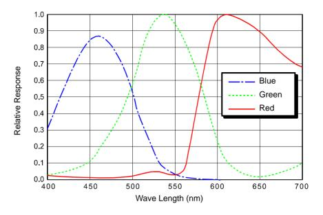
Fig. 16: scA1000-20gc and scA1000-30gc Spectral Response
