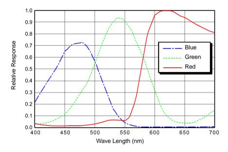
Fig. 19: scA1400-17gc and scA1400-30gc Spectral Response
