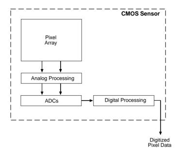
Fig. 34: CMOS Sensor Architecture
