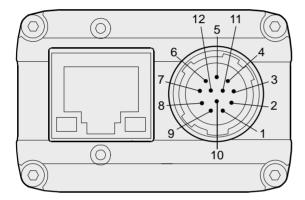
Fig. 37: Pin Numbering for the 12-pin Receptacle
