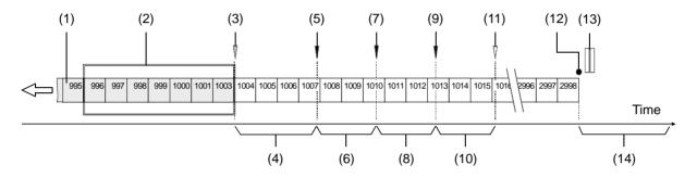
Fig. 29: Incomplete Stream of Packets and Part of the Resend Mechanism
