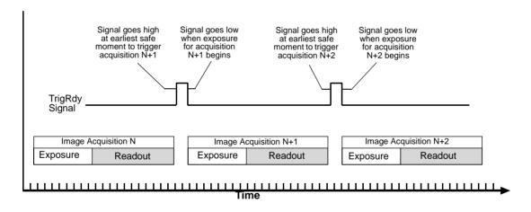
Fig. 52: Trigger Ready Signal
