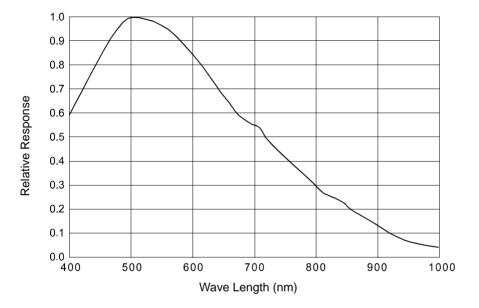
Fig. 1: scA640-70gm Spectral Response Spectral Response
