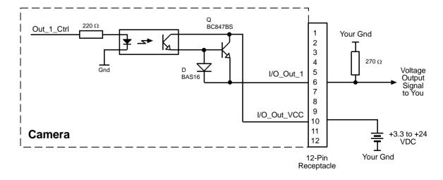
Fig. 40: Typical Voltage Output Circuit
