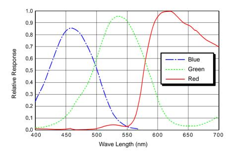
Fig. 20: scA1600-14gc Spectral Response
