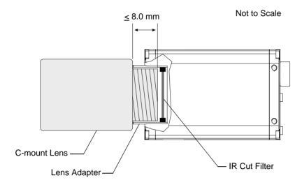
Fig. 27: Maximum Lens Thread Length on Color Cameras
