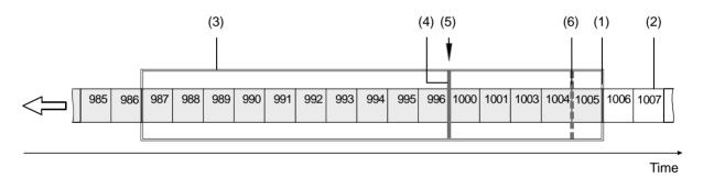
Fig. 28: Example of a Receive Window with Resend Request Threshold & Resend Request Batching Threshold
