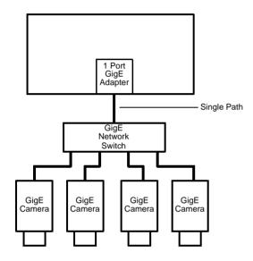
Fig. 31: Multiple Cameras on a Network
