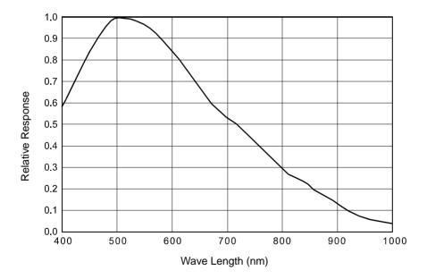
Fig. 5: scA780-54gm Spectral Response
