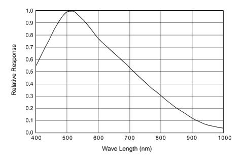
Fig. 8: scA1390-17gm Spectral Response
