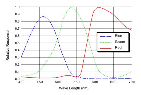
Fig. 18: scA1390-17gc Spectral Response
