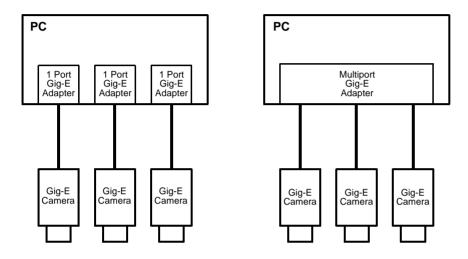
Fig. 2: Peer-to-peer Connections
