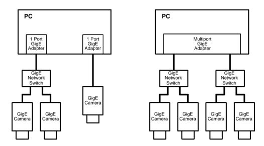
Fig. 3: Network Connections via Switches
