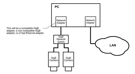
Fig. 1: Network Adapter for the Camera(s)
