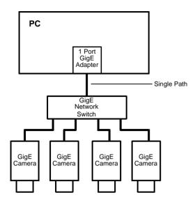
Fig. 4: Multiple Cameras Converging to a Single Path
